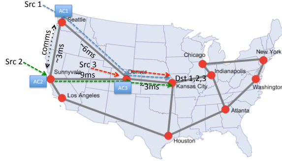
Figure 5: Routing topology used for case study: each source-destination path is denoted by a dashed line. Sources 1 and 2 have edge admission controllers as depicted in Figure 6, whereas Source 3 either has an edge admission controller or an internal admission controller, as depicted in Figure 7, depending on the scenario considered.
